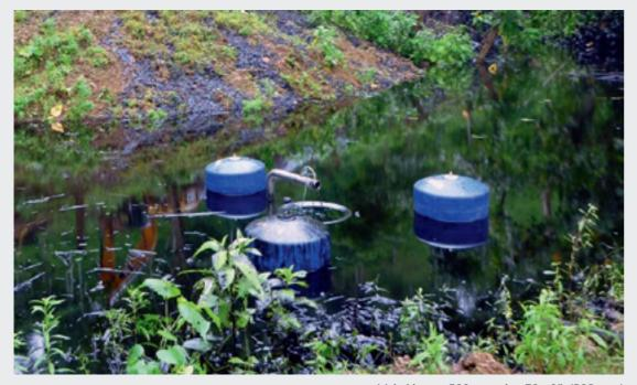
Weirskimmer 500, capacity: 70 m³/h (308 gpm)
