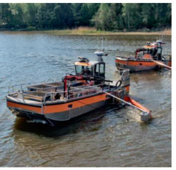
Ultra Shallow Draft Workboat equipped with side cassette for oil recovery
