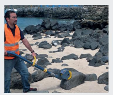
Rock Cleaner (LRC), capacity: 9.7 m<sup>3</sup>/h (43 gpm)
