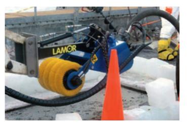
Lamor Recovery Bucket 40 (LRB 40), capacity: 19 m³/h (83 gpm)
