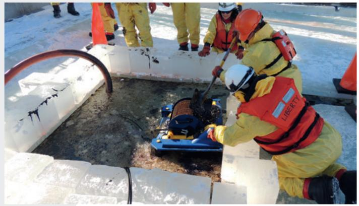
Lamor, a pioneer in oil spill recovery, invented and patented the brush wheel skimmer. This ingenious design is applied in the small portable Lamor Rock Cleaner, in free-floating skimmers as well as oil recovery systems for vessels. Lamor's skimmer portfolio also includes weir skimmers in all sizes and for various applications.
