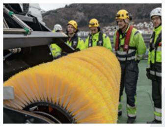
Vessel-mounted Bucket Skimmer (LRB 150), capacity: 115 m³/h (506 gpm)
