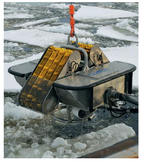
Free Floating 100 (LFF100), capacity: 111 m<sup>3</sup>/h (489 gpm)
