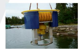
Multiskimmer (LMS 50/70), capacity: 271.5 m³/h (1,195 gpm)
